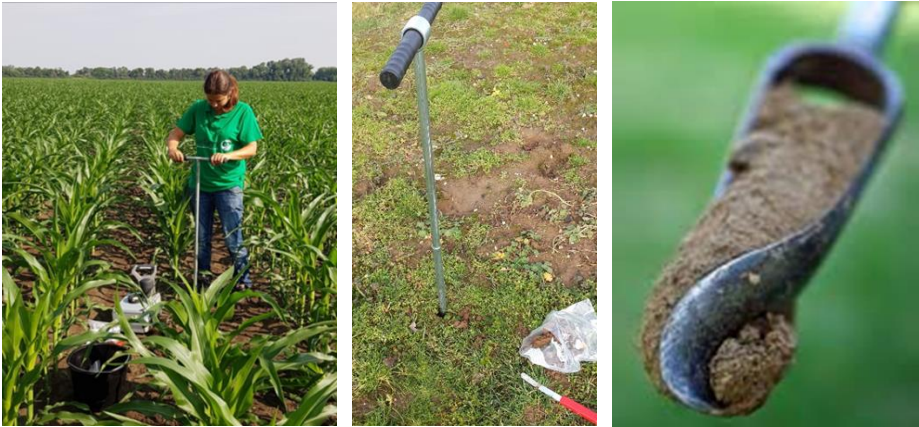
Figure 7: Soil sampling with Eijkelkamp soil auger
