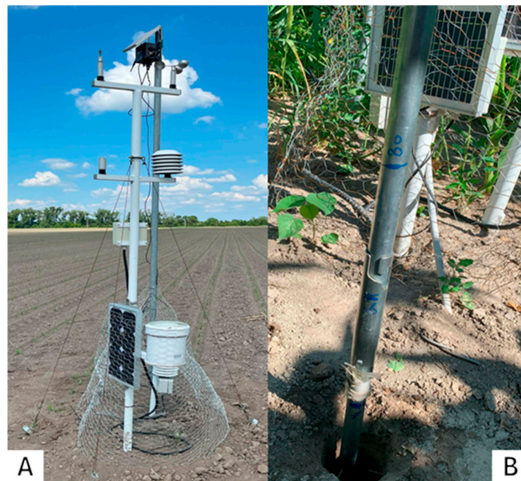
Figure 2. (A) IoT-based meteorological sensor station within the field. (B) Collecting soil samples using a hand auger from sampling points around the sensor stations.
