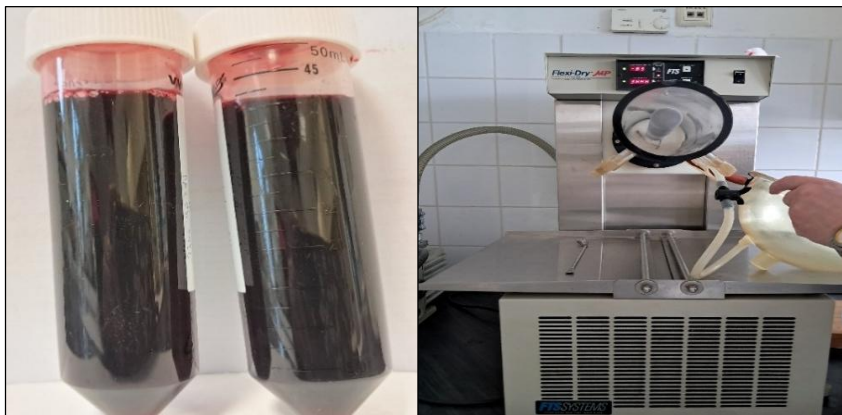
Figure 16 (Left) Glu-LA extract of roselle calyx (30°C for 30 min extraction); (Right) freeze-dryer used for further ENC of roselle extract
