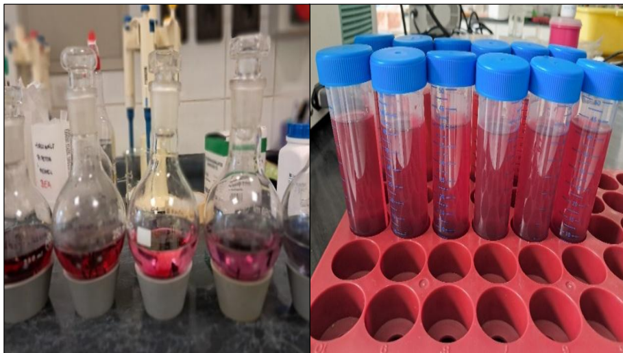
Figure 3 Roselle calyx extracted with 25%, 50% and 75% (v/v) ethanol at varying pH—2.0, 4.5, and 7.0 (Left: extracts after heat refluxing, Right: extracts after centrifuging)
